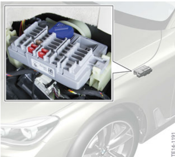
Power distribution box, front left
